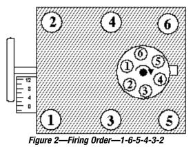
*Rev 9/08 - AJ/mc Brochure #63-2112*  CAMSHAFT: Performer-Plus CATALOG #: 2112 ENGINE: 200-229 c.i.d. Chevrolet 90° V6 RPM RANGE: 1500-5500
